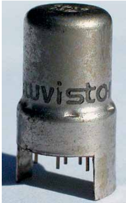
Fig. 7. Nuvistor. These were miniature metal tubes that had usage for the receiving front end stages. RCA announced the first Nuvistor triode tube, the 7586, in 1959. It was intended to be a competitor to the transistor. Height: 0.8 inches, diameter: 0.435 inches. (Bob Kastz, https://wtfamps.com/2018/05/16/the-nuvis-tor-and-bob-katzs-audio-blender-via-inner-fidelity/ )
