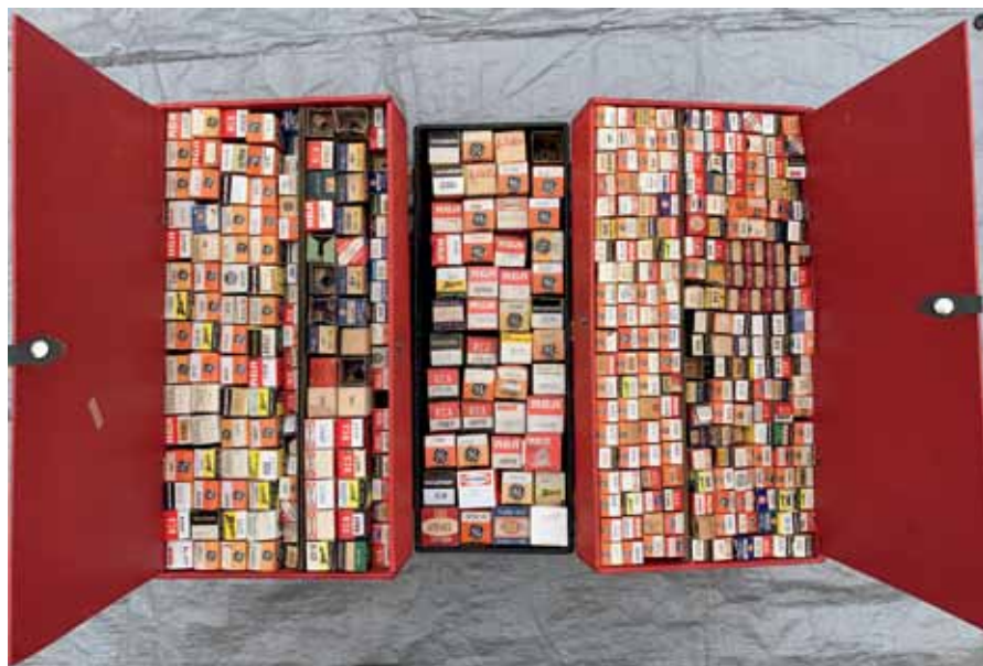
Fig. 13. Tube caddy interior. The bottom part would be filled with tools, and the two parts on the side that fold out would be filled with tubes. A second tube caddy may also be brought along if more tubes were needed. (Author)
