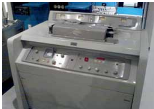
Fig. 11. Ampex VRX-1000 videotape recorder. This was very expensive and could only be afforded by the television networks and the largest individual stations. (Wikipedia photo by Karl Baron from Lund, Sweden)
