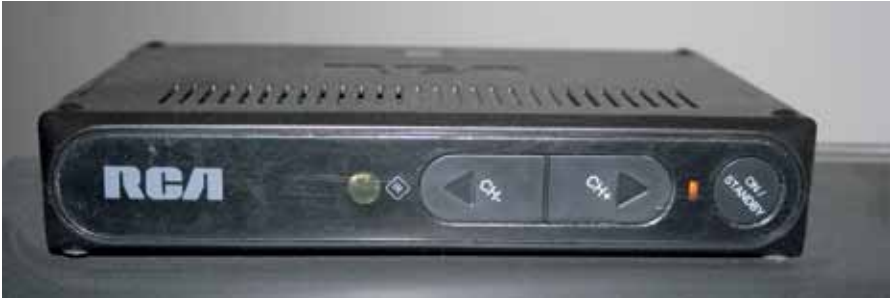
Fig. 8. Digital TV converter box. This was a short-lived product as TVs were quickly bought new with only the digital tuners. (By Jeffrey Beall - own work, CC BY-SA 3.0, https://commons.wikimedia.org/w/index.php?curid=4973347 )
